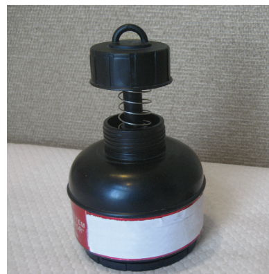
Figure 3 – Long-Term Electret Ion Chamber
